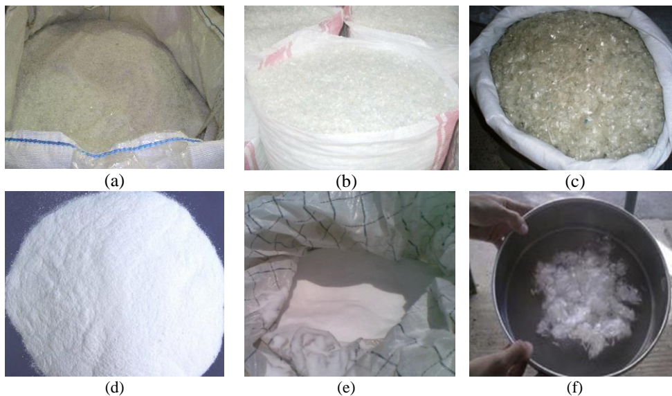
Fig.1 (a) Pulverized Polyethylene Terephthalate (b) Granulated Polyethylene Terephthalate (c) PET flakes (d) Low Density Polyethylene Powder (e) High Density Polyethylene Powder (f) Polypropylene fiber
